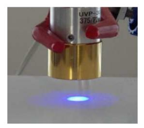
[ Power: 3.6v-25mA ] A manually variable power supply, with an output regulated to 25mA. Rated point diameter can be visually confirmed.
